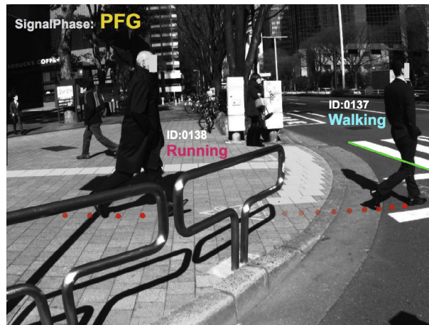
Fig. 5. Image example of the manual labeling. The red points are the labeled grounding points of the pedestrians. The green line is the edge line of the crosswalk. The pedestrian motion type and signal phase (with the other cameras) are also labeled manually. (For interpretation of the references to color in this figure legend, the reader is referred to the web version of this article.)
